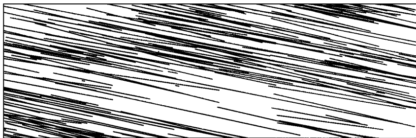
FIG. 8. Fracture realization generated using statistics from the Mesaverde fracture system presented in Table 2.
